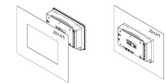
2. Insert the panel mount brackets into the bracket mounting holes as shown in the image below, pulling the bracket to lock it into place.
