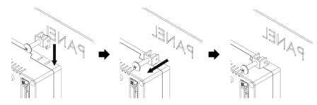
3. Tighten the bracket mounting bolts to secure the display to the panel. The recommended torque is  $0.4\ Nm.$
